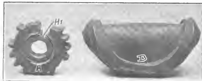
Fig. 7—Materials of which the gears are made after they were subjected to a test of destruction
